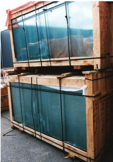
Figure 5: Heavy glass corrosion after transport under unfavourable climatic conditions; high humidity, extreme temperature changes.
