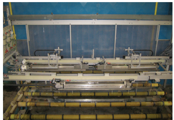
Figure 7: The Liquid Applicator, installed on a float line.
