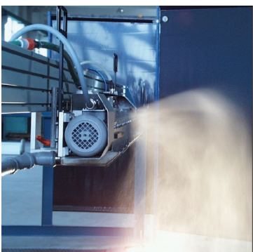
Figure 6: The Grafotec Liquid Applicator produces a spray 'curtain' that covers the glass surface with AC Resistain TC.
