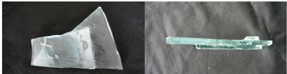
Figure 2: Glass corrosion in the end state; heavy, white staining, destacking not possible without breakage.
